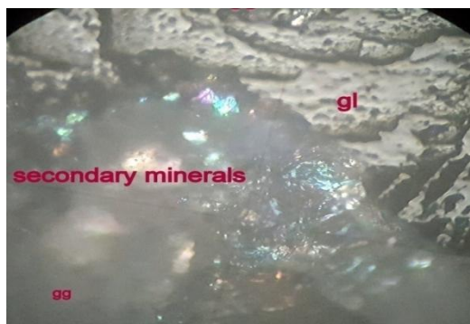
Plate 5: Photomicrograph showing galena at the area. gl = galena, gg = gangue. Note the replacement at the edges of galena by secondary minerals which include cerussite, anglesite, chalcocite and malachite (ppl x1.25 \mu m).
